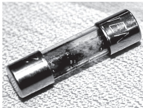
This is a blown fuse, notice the discoloration inside the glass part.
